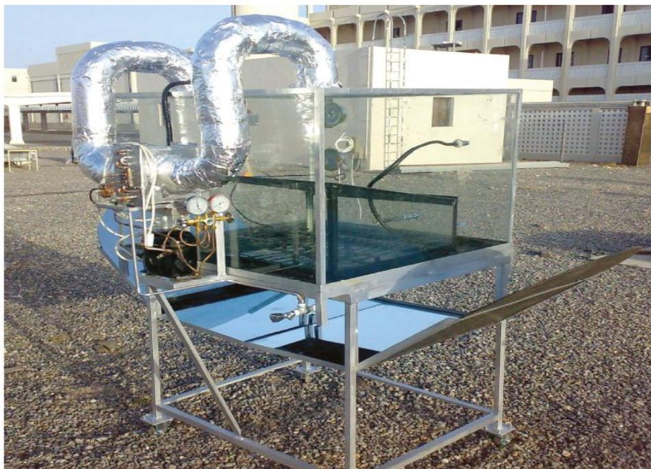
Fig.8: Experimental setup of an inverted absorber solar still with a refrigerator cycle by Abdul-Wahab and Al-Hatmi [42]
