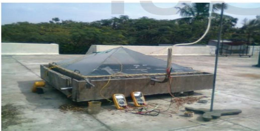
Fig.2: Experimental setup of a tilted-wick type solar still with pyramidal glazing by Prakash et.al. [18]
