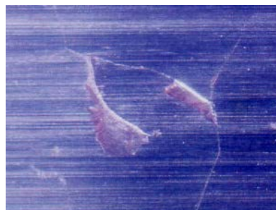
Figure 6. Small holes on the surface of the rollers
