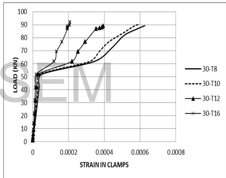
Figure (8) Strain in Clamps of Specimen with  $f_{cu}=30\text{N/mm}^2$
