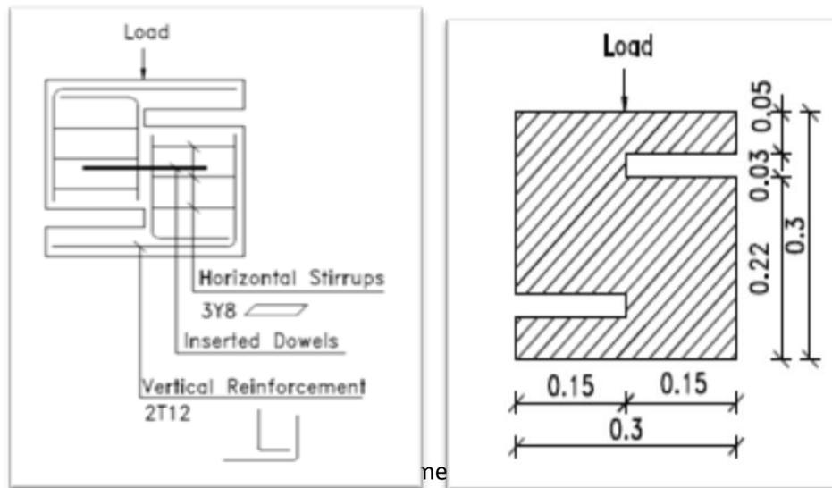
Figure (2): Specimen Dimensions & Reinforcement
