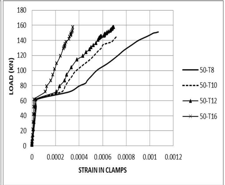
Figure (10) Strain in Clamps of Specimen with  $f_{cu}=50\text{N/mm}^2$
