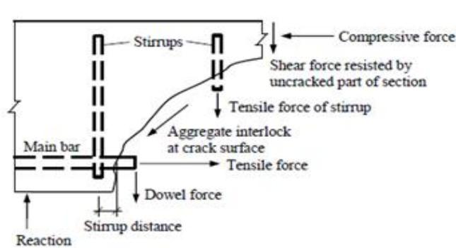
Figure (1): Internal Forces in Cracked Beam
