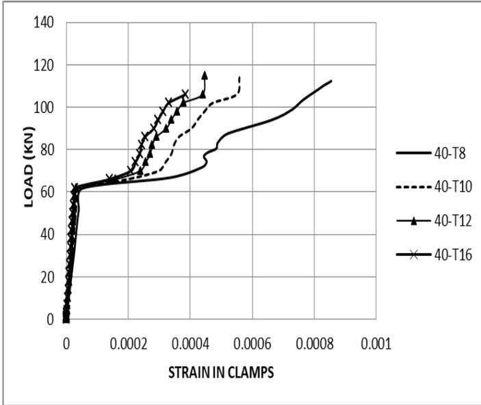
Figure (9) Strain in Clamps of Specimen with  $f_{cu}=40\text{N/mm}^2$
