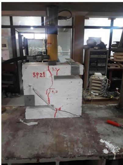
Figure (9): Crack Profile for Specimen in In Group (G)
