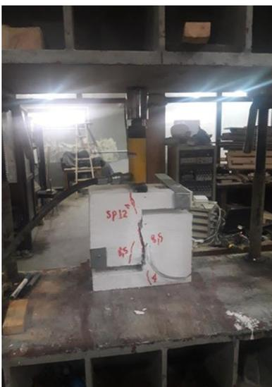
Figure (6): Crack Profile for Specimen in Group (D)
