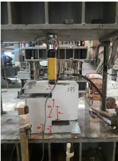
Figure (3): Crack Profile for Specimen in Group (A)
