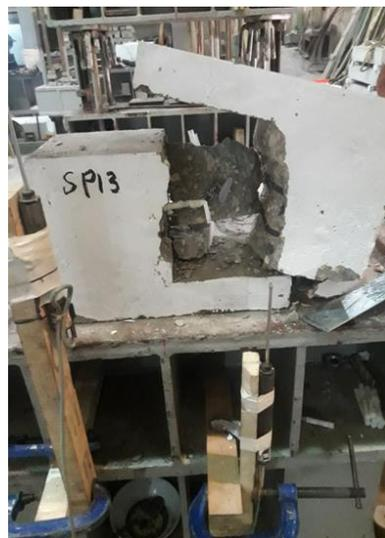
Figure (7): Crack Profile for Specimen in Group (E)
