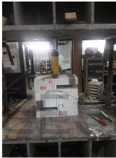
Figure (4): Crack Profile for Specimen in Group (B)
