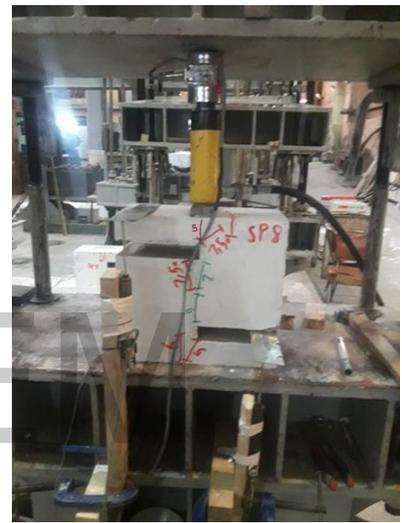
Figure (5): Crack Profile for Specimen in Group (C)
