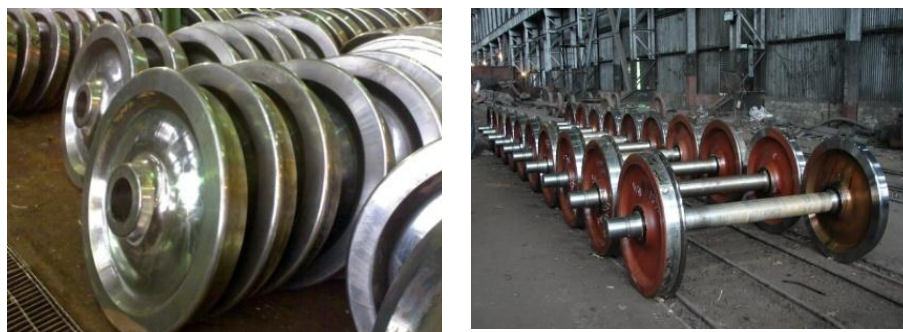
Fig.10 Tested OK loose wheel and assembled wheel sets ready for despatch
