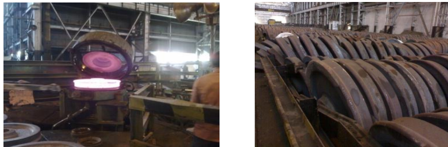
Fig.8 Heat Treatment of wheel and stacking of Heat Treated black wheels
