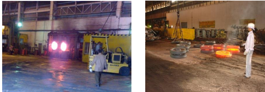
Fig.5 Rolling of wheel in Wheel Mill and final wheel after forging
